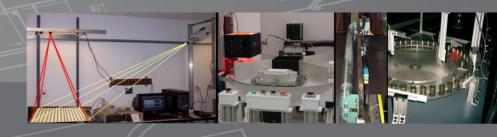
a machine at a rate of 450-600 parts per minute are inspected by a high resolution camera. Due to the process engineers configure various programs to inspec sizes, holes, shape
